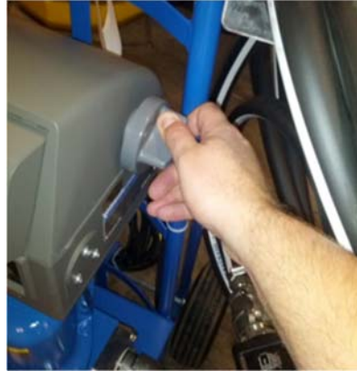
B. Turn reset knob to set register to zero and lock ticket into place.
