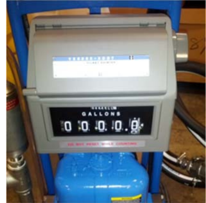
B. Turn reset knob to set register to zero and lock ticket into place.
